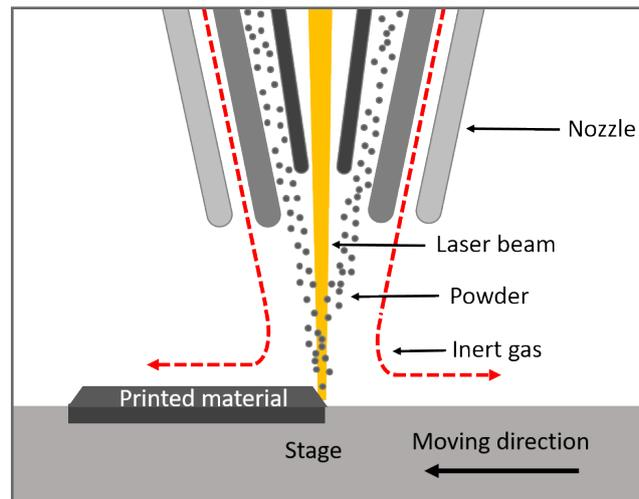
Figure 1: process of additive laser powder build-up welding.
