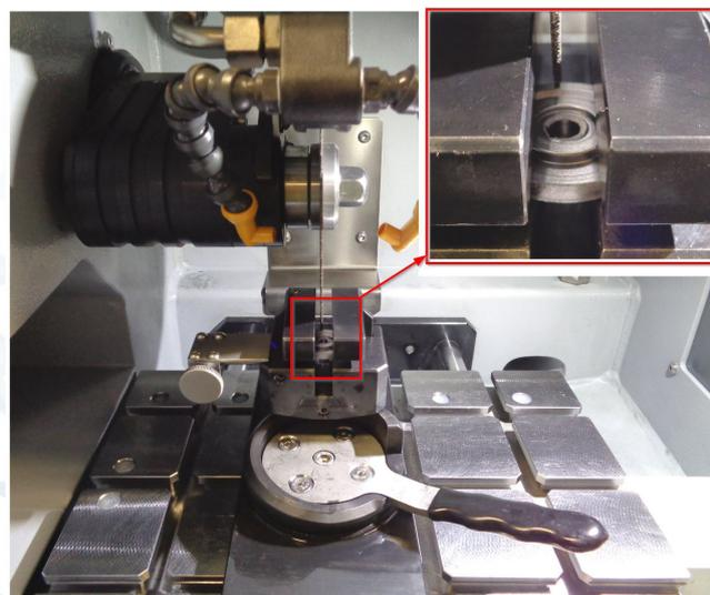
Figure 2: Brilliant 220 machine setup. Detail: clamped sample (clamping tool: vertical vice single).
