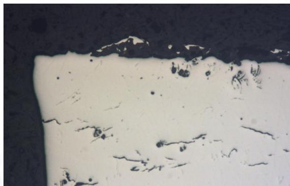
Figure 3: Image of the prepared specimen surface. Due to the polished surface the light is reflected almost equally and the microstructure is not discernible.
